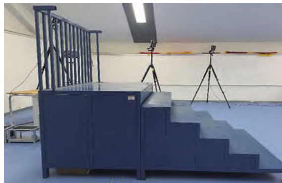
图 1 模拟楼梯 Fig.1 Simulated staircase
